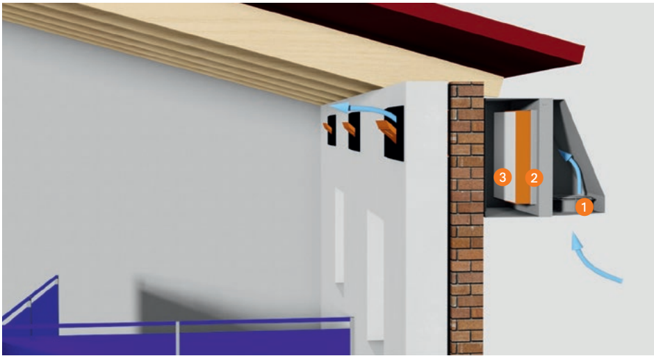
Functional diagram of the APT 1500 for decentralised fresh air guided by the CL 1200 fresh air inlet
